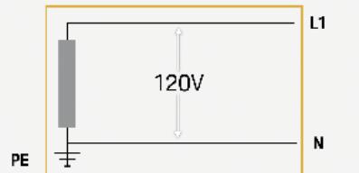
Fig. 7: Network configuration, single phase 120 V two-wire grid variant with earthed N-line and  $I_{max} = 80 \text{ A}$
