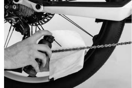
Figure 21: Lubricating the chain
