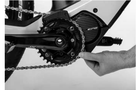
Figure 22: Checking the condition of the chain
