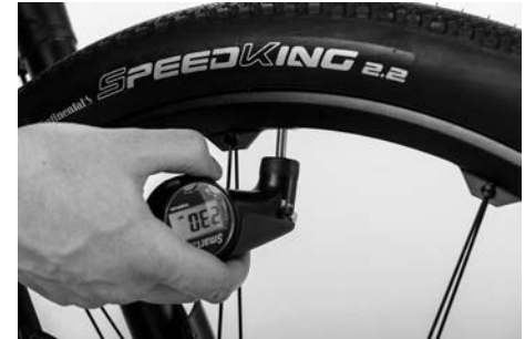
Figure 12: Checking the tyre pressure.
