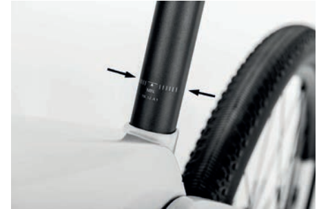
Figure 39: Seat post (maximum extension length).
