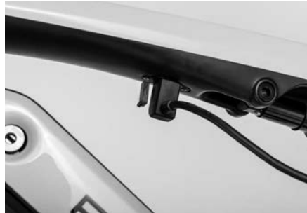
Figure 27: Charger cable in the correct position
