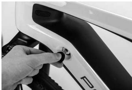
Figure 29: Operating the removal mechanism
