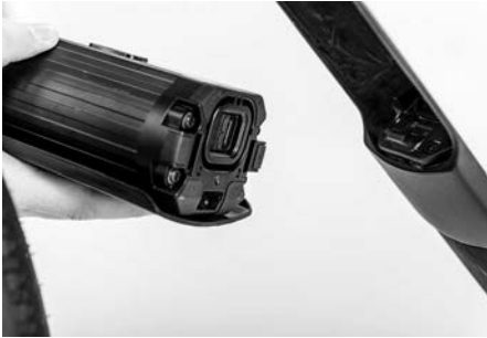
Figure 32: Installing the drive battery
