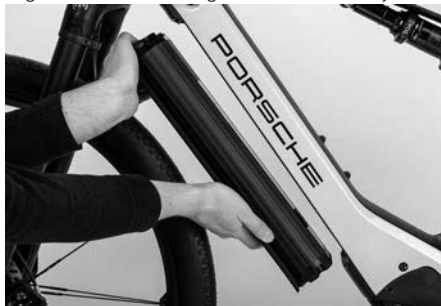
Figure 31: Removing the drive battery
