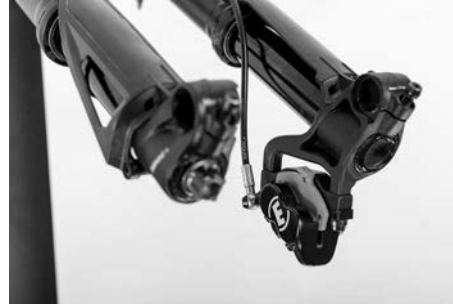
Figure 64: Transport guard for the disc brakes
