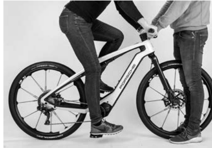
Figure 38: Identifying the correct saddle height.
