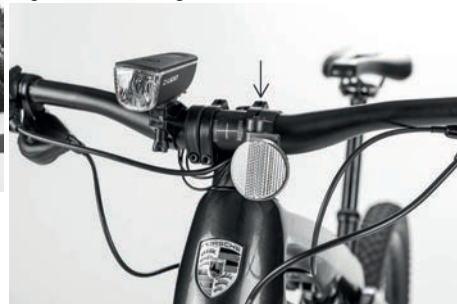
Figure 62: Fitting the front reflector
