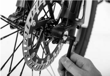
Figure 50: Fitting the safety cover
