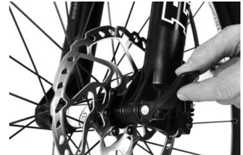
Figure 53: Fitting the Cross front wheel axle system
