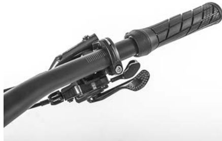
Figure 24: The position of the shifting lever (electronic)
