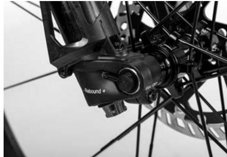
Figure 52: Inserting the breakdown tool
