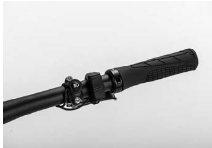
Figure 24: The position of the shifting lever (electronic)
