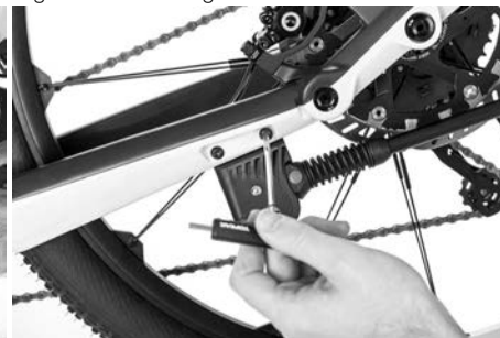
Figure 57: Fitting the stand
