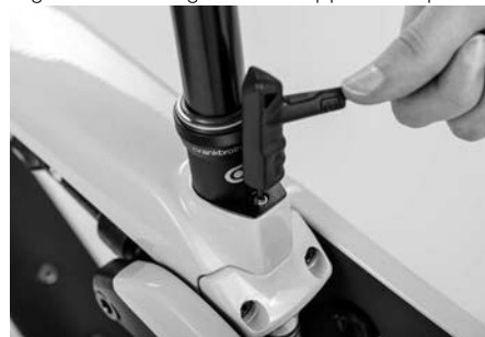
Figure 42: Wedge bolt/Dropper seat post
