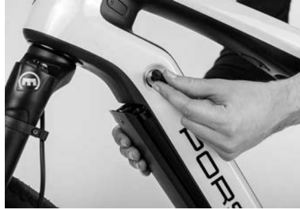
Figure 33: Securing the drive battery
