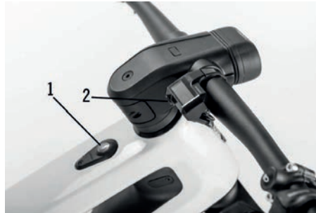
Figure 5: On/off button (1) and display button (2)
