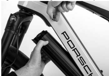
Figure 31: Removing the drive battery
