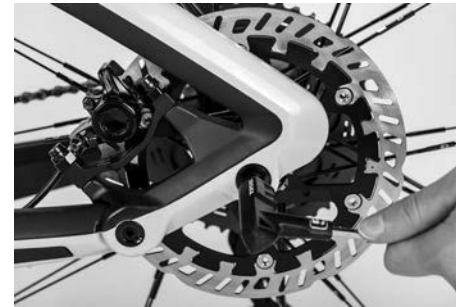
Figure 54: Fitting the rear wheel axle.
