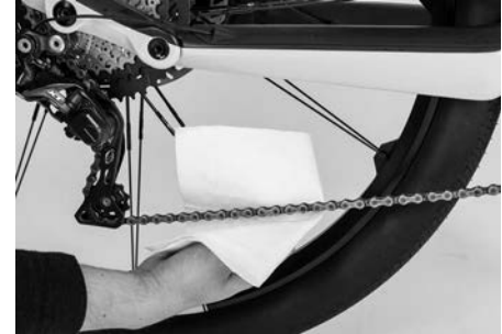
Figure 21: Lubricating the chain
