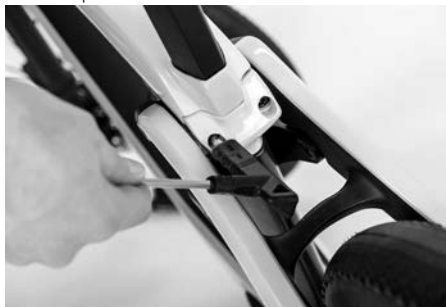
Figure 40: Clamping screws/AERO seat post
