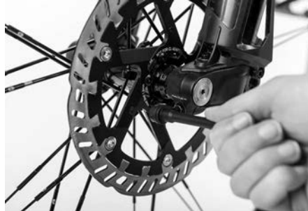
Figure 52: Inserting the breakdown tool
