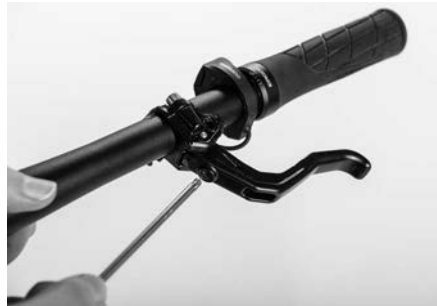
Figure 19: Brakes / grip width
