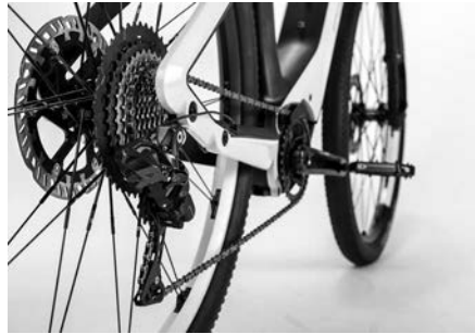
Figure 18: Chain on the chain ring/cassette
