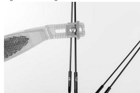
Figure 60: Fitting the side reflectors
