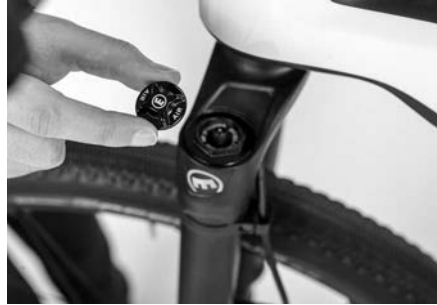
Figure 43: Valve for adjusting the fork pressure.
