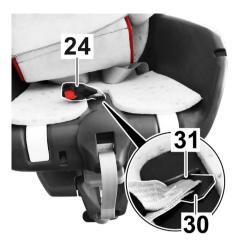
Push the Triglide (30) with which the buckle (24) is fastened to the seat shell upright through the belt slot (31).
