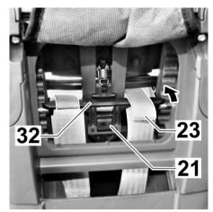
11.Tilt the headrest forward and push the belt loops of the shoulder pads (23) onto the bridge (32) of the headrest adjuster (21).
